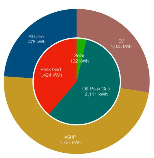
Outer Circle Total Electricity Usage Split By Energy Destination 3,667 kWh
